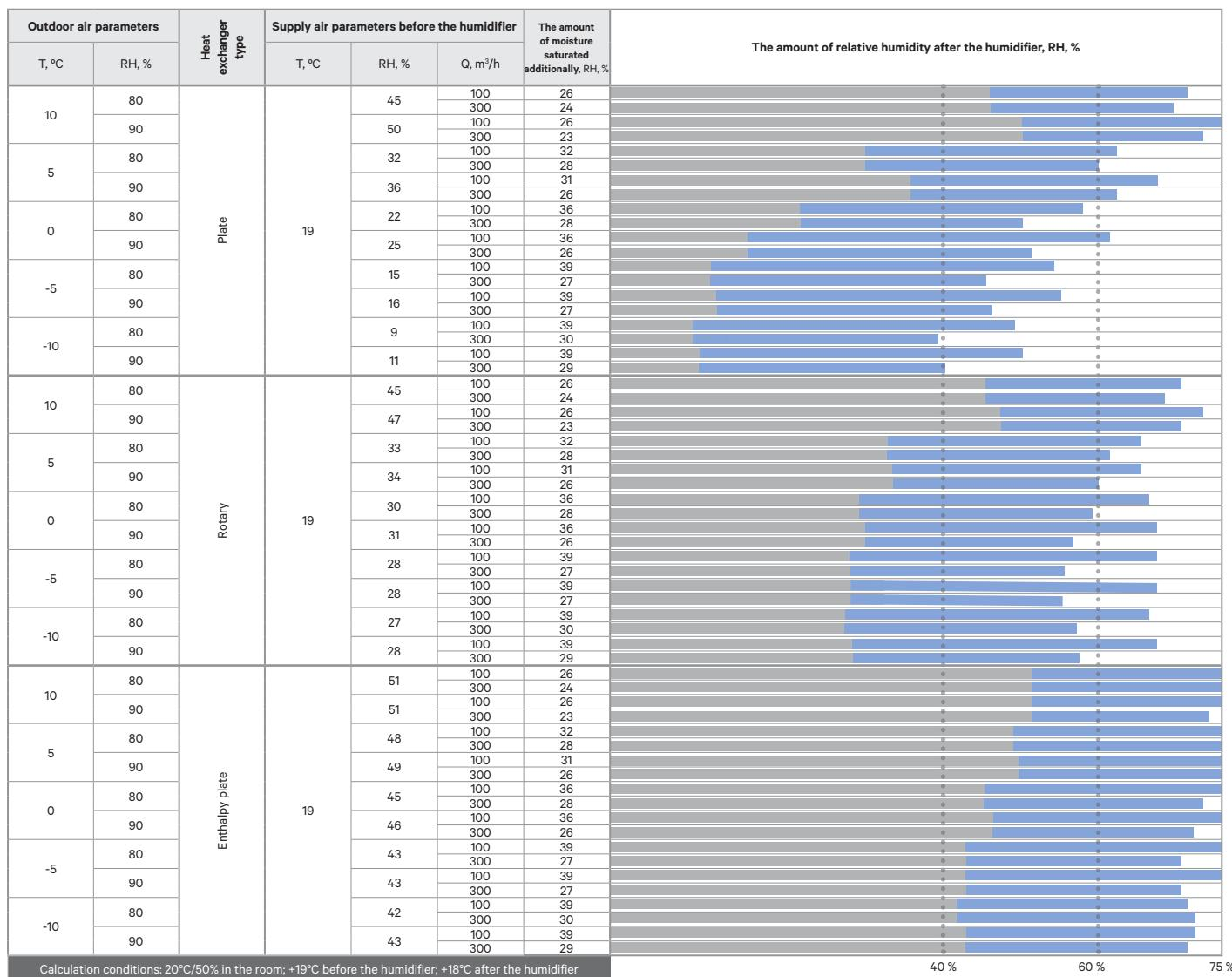
Note: when the amount of relative humidity after the humidifier is up to 75%, the intensity of humidification automatically reduced.
