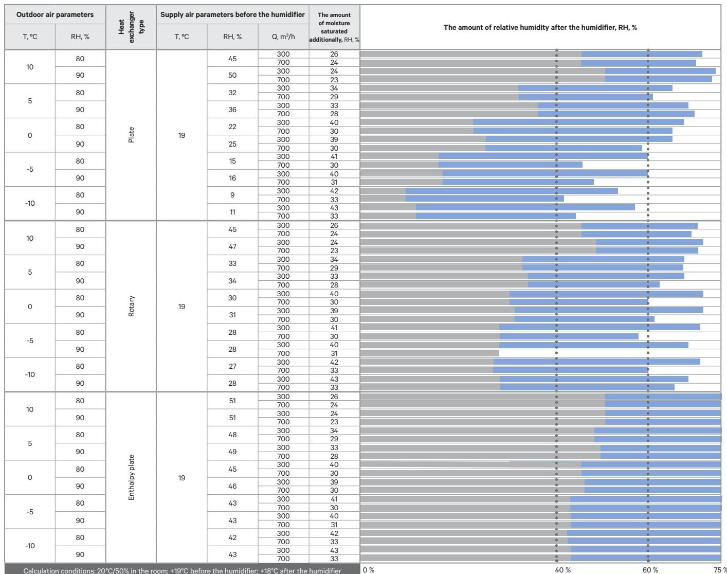
Marking: T, °C air temperature; RH, % relative humidity; Q, m<sup>3</sup>/h air quantity.
